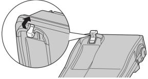
$2 \begin{tabular}{ll} $$ Press the tabs in the direction of the arrows ((1)), then remove the wall mounting adaptor ((2)). \end{tabular}$
