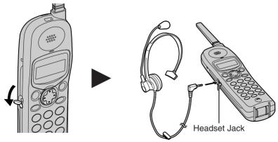
To switch to the speakerphone while using the headset: Press 健. To return to the headset, press ♪.
